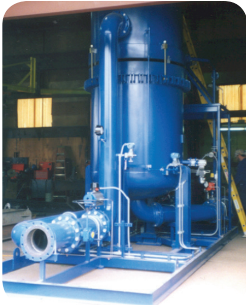
1000 ft 2 backwash filter skid
