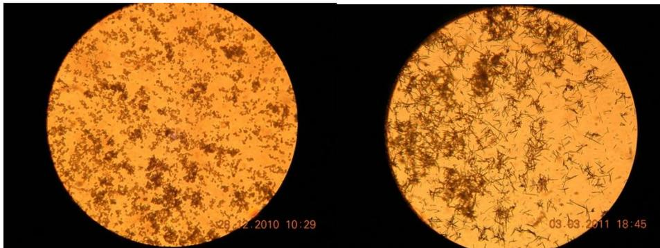
**Figure 9: Crystals formed by untreated water (left) and treated water (right)**
