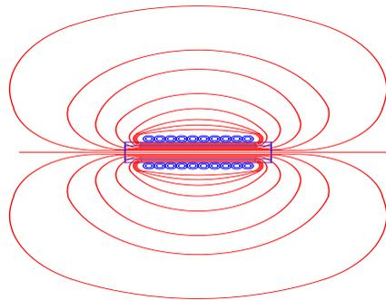
Figure 2: Magnetic field lines produced by a non-intrusive electromagnet
